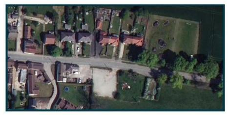
Utilities enquiries have been carried out along with a topographical survey which indicates that consideration needs to be taken in regards an easement for a pumping station and also relocation of a telegraph pole. A provisional sum has been included for this.
